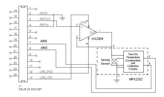
Since the excitation voltage is 2.5V, the full span output is scaled to 10mV. When the input of the EMANT300 is set to this range, the module can measure better than 1uV due to its programmable gain amplifier and the resolution of the ADC.
