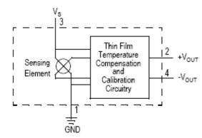
The differential voltage output of the sensor is directly proportional to the differential pressure applied. The absolute sensor has a built-in reference vacuum. The output voltage will decrease as vacuum, relative to ambient, is drawn on the pressure (P1) side. The output voltage of the differential or gauge sensor increases with increasing pressure applied to the pressure (P1) side relative to the vacuum (P2) side.
